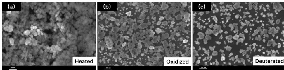
**Fig. 1.** SEM of PNZ7 after (a) High-temperature vacuum, (b) Air calcination and (c) High-temperature deuterated.
