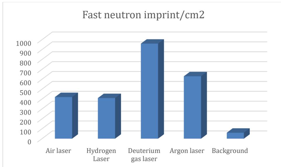
Figure 1: Number of neutron imprints produced by laser irradiation on titanium metal in different gas atmospheres
