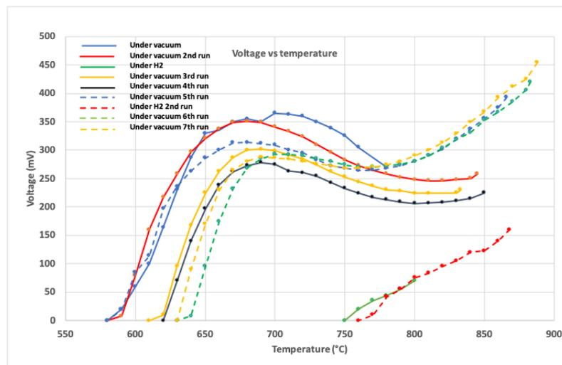
Figure 1: Voltage between an electrode composed of Ni/Cu nano-powder and a stainless-steel counter electrode. The voltage varies with the various cycles of loading and de-loading. The voltage is higher under vacuum.
