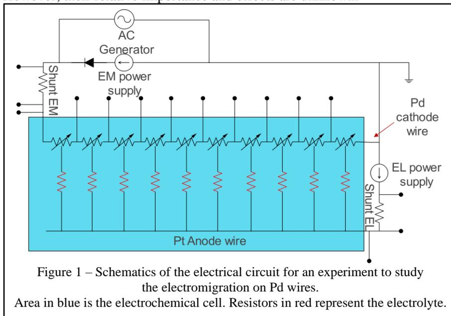
We designed a new experiment to measure the directions and magnitudes of electromigration in Pd wires that are 250  $\mu\text{m}$  in diameter and 10 cm in length. Using knotted Pt wire leads, we have contacts to the wire with separations of 1 cm. The Pd wire is the cathode in an electrochemical cell in which the anodes are separate 1 cm-long Pt wires near each of the Pd segments. This arrangement enables us to load protons into
