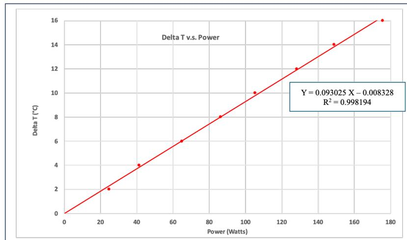
Calibration of the No-Loss Airflow Calorimeter for a constant air mass flowrate of  $0.0105 \text{ kg s}^{-1}$  – The linear relationship between the power and the air temperature shows that all the heat is captured by the airflow and no heat is lost to the environment.
