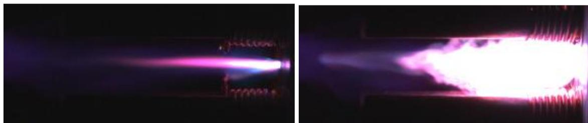
Figure 1. Detonation in hydrocarbon heterogeneous plasma. Right- metastable heterogeneous plasma (carbon nano-clusters+ hydrogen ions). Left- time moment of ignition of this plasma
