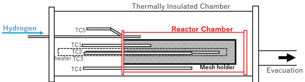
Fig.1: Schematic of the experimental setup.
