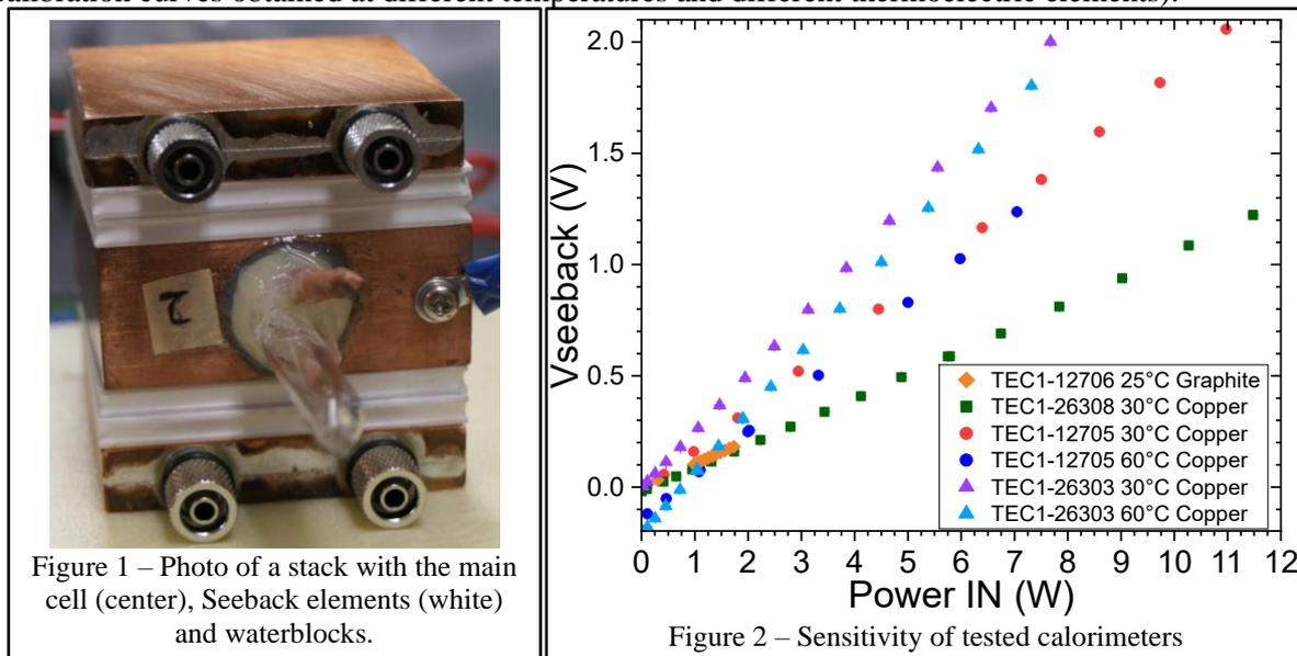
The response of the calorimeter is very linear, highlighting very small heat losses.
