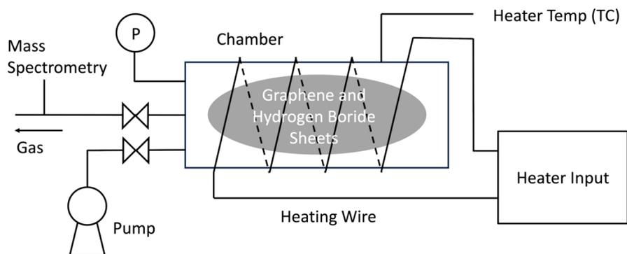
Fig. 1 Hyper-Cold Fusion Experimental Setup
