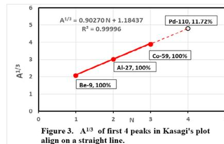
Figure 3.  $A^{1/3}$  of first 4 peaks in Kasagi’s plot align on a straight line.
