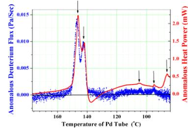
Figure 1. Correlation between anomalous D<sub>2</sub> flux peaks and anomalous heat power peaks while Pd tube is cooling down
