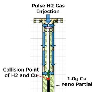
Fig.1 Chamber of new reaction system
