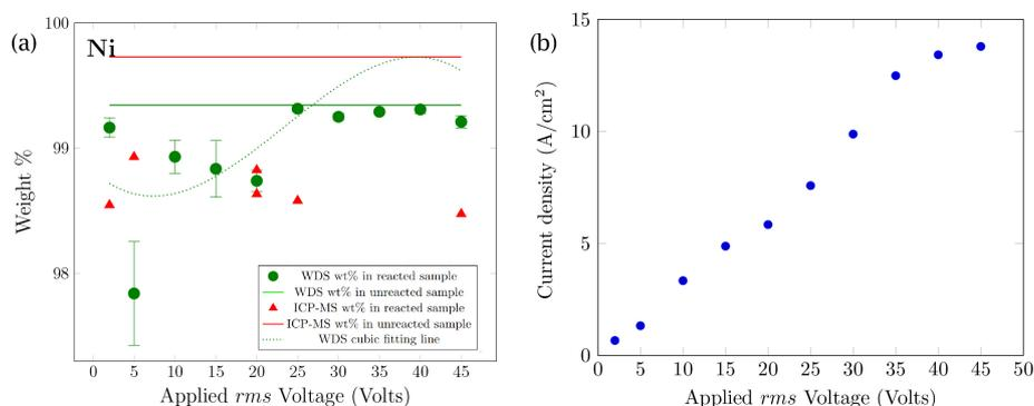
Figure 1: (a) Plots show Ni wt% data from WDS (green circles) and ICP-MS (red triangles). Horizontal lines indicate unreacted sample wt% for comparison, and the green dotted line is the cubic fit for WDS data. (b) V-I characteristics of electrolytic cell
